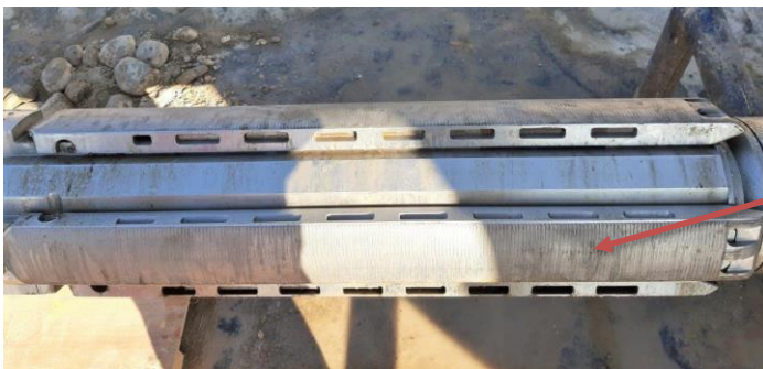
VectorZIEL RSS steering unit after a 200-hr run
