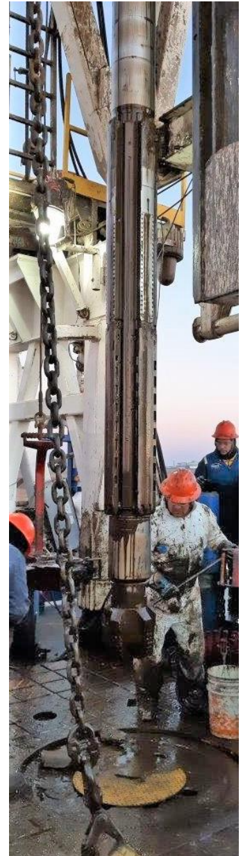
VectorZIEL RSS steering unit after a 200-hr run
