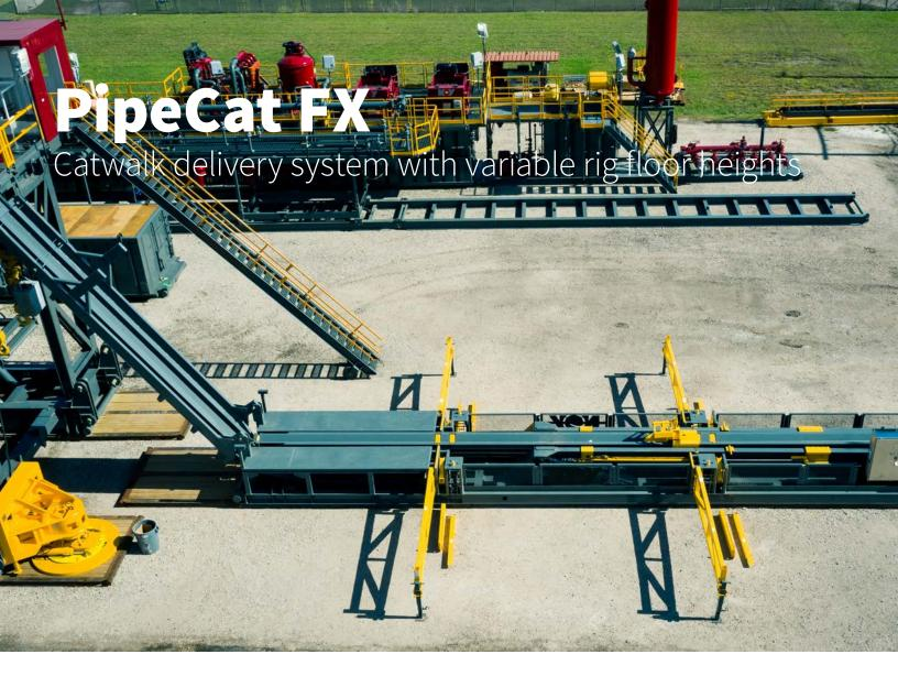
The PipeCat™ FX delivers tubulars from the ground level to the drill floor and back. The adjustable catwalk can accommodate floor heights from 25 to 38 ft. Capable of handling Range 2 and Range 3 tubulars with diameters from 3.5 to 20 in., the tool has a lifting capacity of up to 10,000 lbs.
