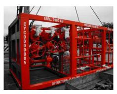
**10k/15k wellhead desanders:** High pressure cyclonic desanders for solids removal from multiphase fluids
