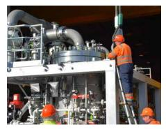
**ToreTrap:** Cyclonic produced water desanders for removal of solids down to 10 micron
