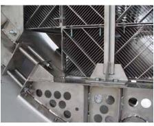
**Plate packs:** Vessel internals for removal of fine solids and oil droplets
