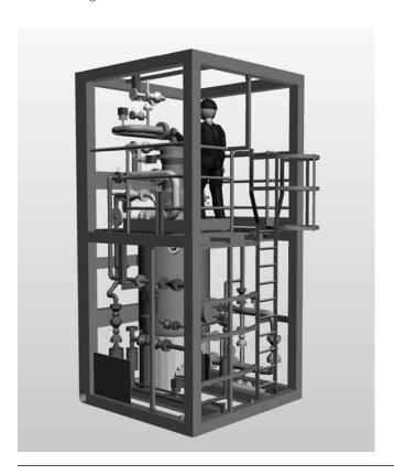
vessel, through the jet pump, to the single cyclone section, and back into the accumulator. The sand is circulated around this circuit for a predetermined time or until a sample indicates the sand has reached the required standard.
